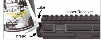
5 Test fit barrel nut on the upper receiver by hand tightening it on, then remove.
