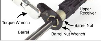
(8) Loosen the barrel nut one-half turn and re-torque to 45 ft-lbs (Do not exceed 50 ft-lbs).
