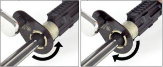
Install the gas block & gas tube.
